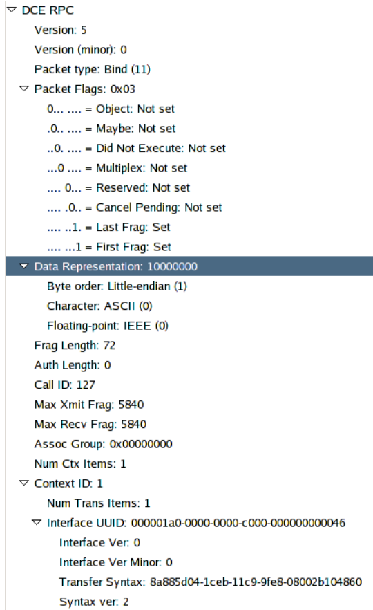
Figure 21: RPC bind request sent by the oc192-dcom tool
